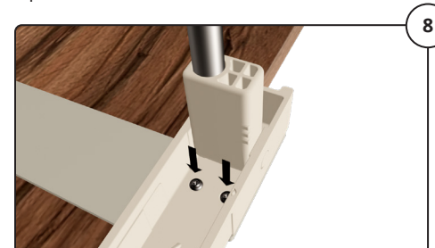
Tighten the inner screws (M3x8) (on both sides).
