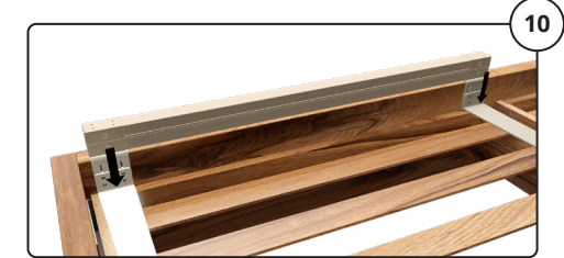
Place at the edge of the bed and adjust the height of the angle. The visible screws can now be tightened.
