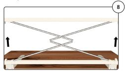
Screw in the remaining screws and tighten all screws (do not overtighten).
