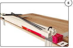
Put on the outer screws (do not tighten). Repeat on the opposite side.
