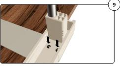
Place the cross connector with the markings on the topside on the table.
