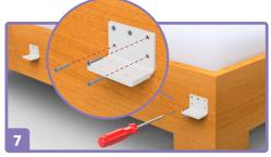
Secure both brackets with remaining screws.
