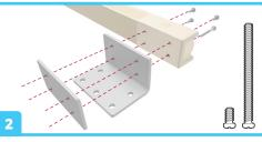
Attach both brackets with thread plate on the AIRZAG using 4 screws each.
