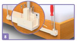
Mount AIRZAG again. Fasten with four screws each.
