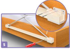
Open AIRZAG and screw on with two screws each.
